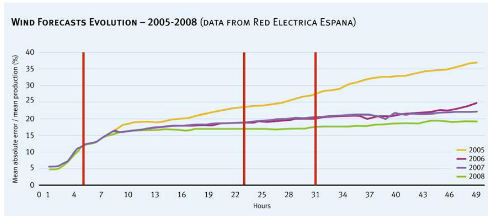
Figure 2: Evolution of the wind forecast error, as a percentage of wind production, as a function to the distance to real time. Source: (EURELECTRIC, 2010).
